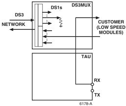
Figure 575-3a. Drop: None/Insert: Network
